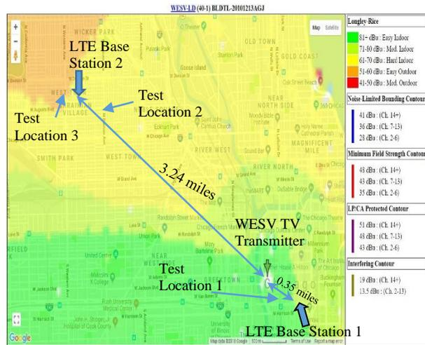
FIGURE 7: FIELD TEST LOCATIONS FOR LTE DOWNLINK.
