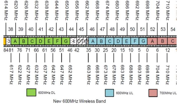
FIGURE 1: LTE DOWNLINK, UPLINK AND CORRESPONDING TV CHANNEL FREQUENCIES.
