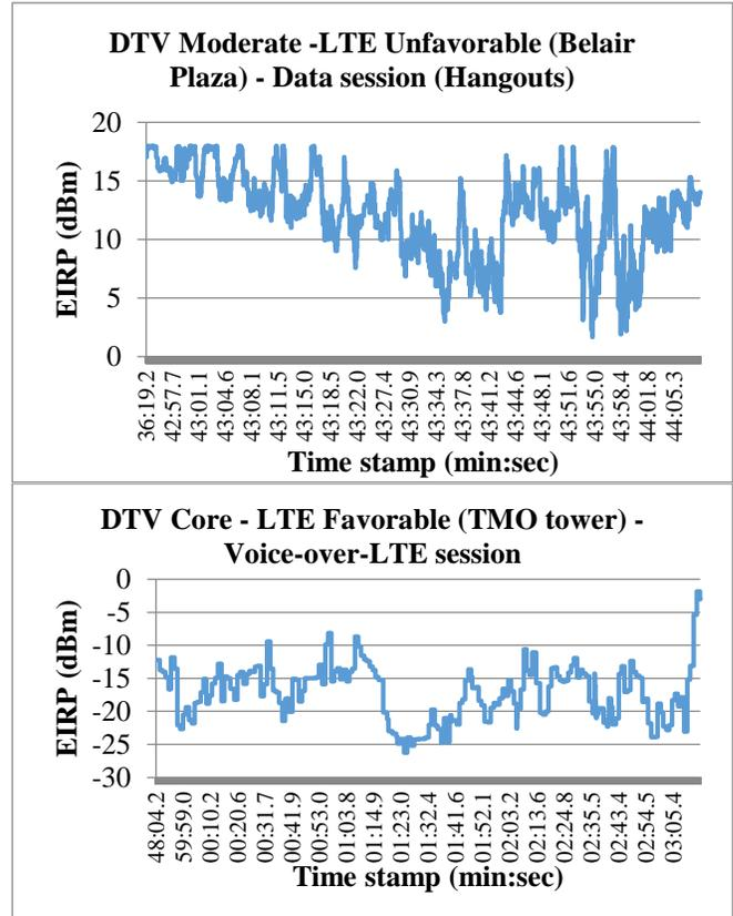
FIGURE 10: TRANSMIT POWER MEASUREMENTS FROM UE
