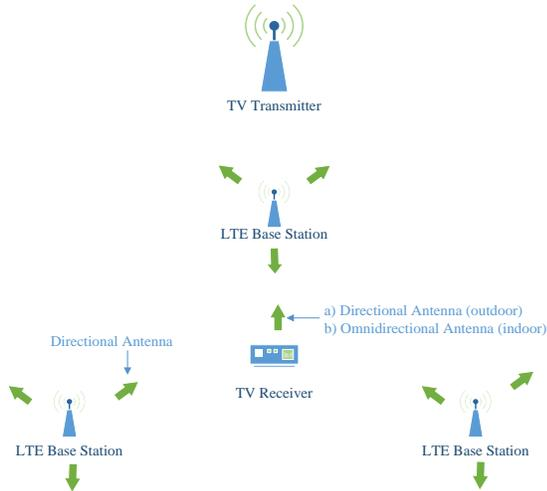
FIGURE 2: INTERFERENCE MECHANISM FOR LTE DOWNLINK.
